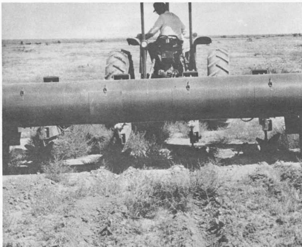
KIMSEED Seeder — This type of seeder modifies the microclimate by cutting interrupting furrows that act as water trapments, which holds soil moisture for good grass seed germination. The KIMSEED seeder is an Australian design.
