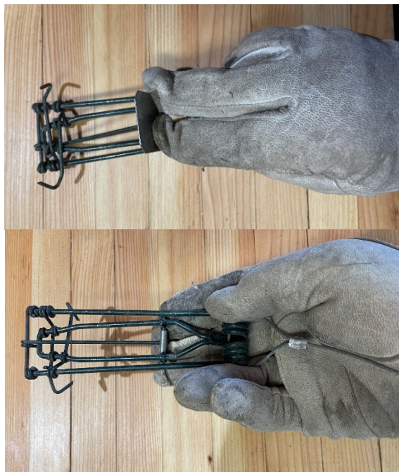
Figure 6. Hold the trap to keep the pan from firing while placing the trap.
