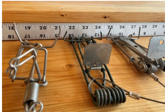
Figure 7. Jaw widths of set traps range from about 2 1/2 to 3 inches across or about the average size of a pocket gopher tunnel.
