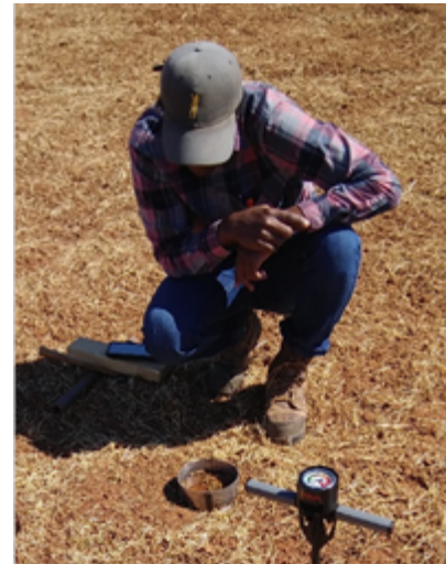
Measuring water infiltration rates and soil compaction to 24"
